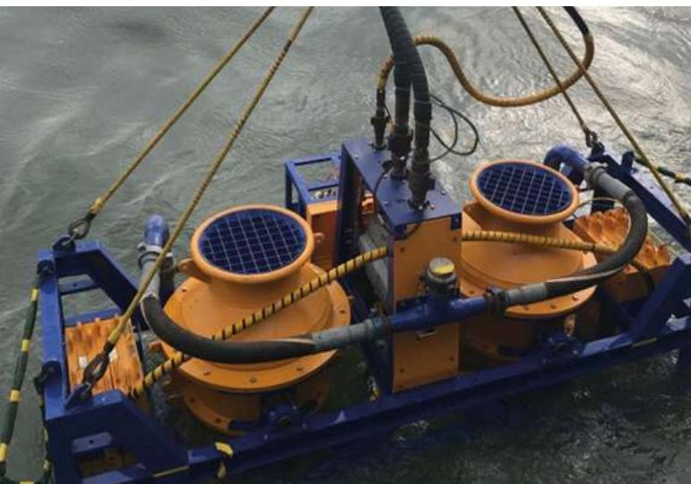
During CFE operations, Gemini NBI sonars were used for real time imaging. Gemini data was logged with screen grabs taken at intervals agreed with the client. CFE operations were conducted using the vessel starboard crane, deploying over the starboard side. The vessel speed during operations was 2 - 3 m/min.
